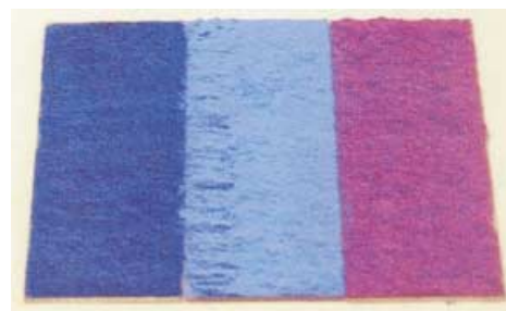
Figure 2. Egyptian Blue ( \text{CaCuSi}_4\text{O}_{10} ; left), Chinese Blue ( \text{BaCuSi}_4\text{O}_{10} ; middle), and Chinese Purple ( \text{BaCuSi}_2\text{O}_6 ; right). Egyptian Blue and Chinese Blue appear very similar under comparable conditions. That they appear different here is a result of the samples being of different particle size. Small particles lead to lightening in tone. The sample of Egyptian Blue consists of coarse crystalline material, while Chinese Blue was ground.
