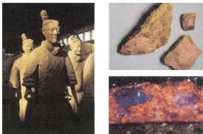
Figure 1. Sample of the Terracotta Army Xi'an, China. Left: a group of terracotta soldiers. Top right: fragments of the purple trousers of a soldier (fragment 003–92). Bottom right: A microscopic view (enlargement 500-times) of a cross section of its pigment layer. The displayed part has a horizontal extension of 0.22 mm. The pigment layer contains grains of Chinese Purple and Cinnabar. Under the pigment layer there is a dark lacquer and under that the terracotta.
